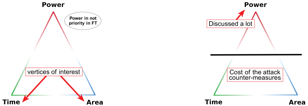
Figure 2: Comparison of system design approaches (vertices of interest) in the field of fault tolerant and attack resistant systems. On the left the triangle illustration of the fault tolerant system shows the need to implement redundancy by using area and time resources of the system to add some fault tolerant properties. The triangle illustration on the right on the contrary points that in the field of attack resistant systems the power consumption is discussed a lot as it can reveal secret information to the attacker.
